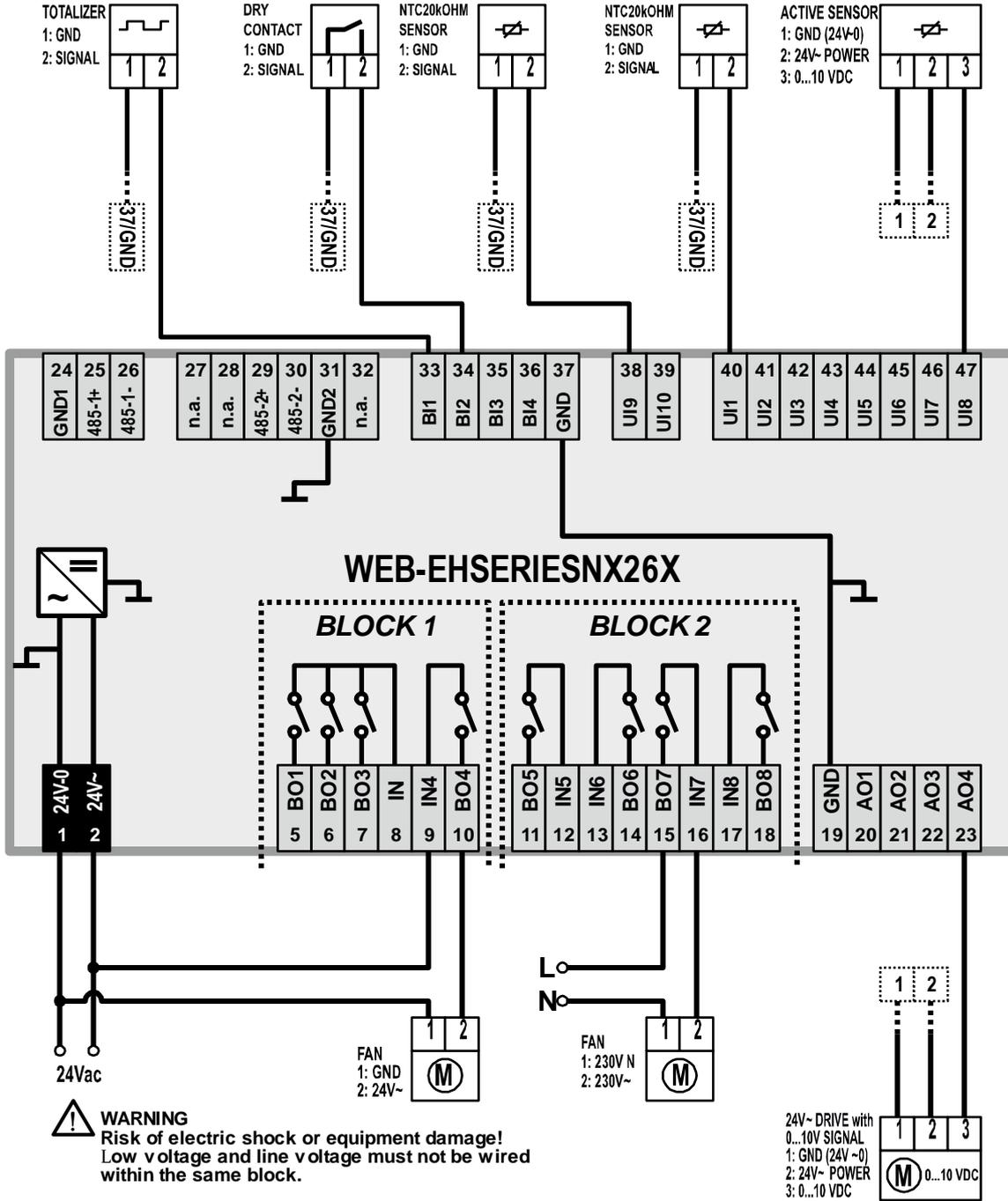
Figure 28: WEB-EHSERIESNX26X connection example
