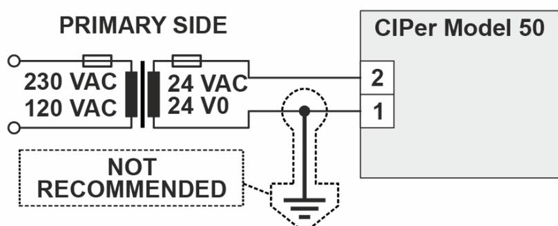
**Figure 25: Connection of CIPer Model 50 controller**
