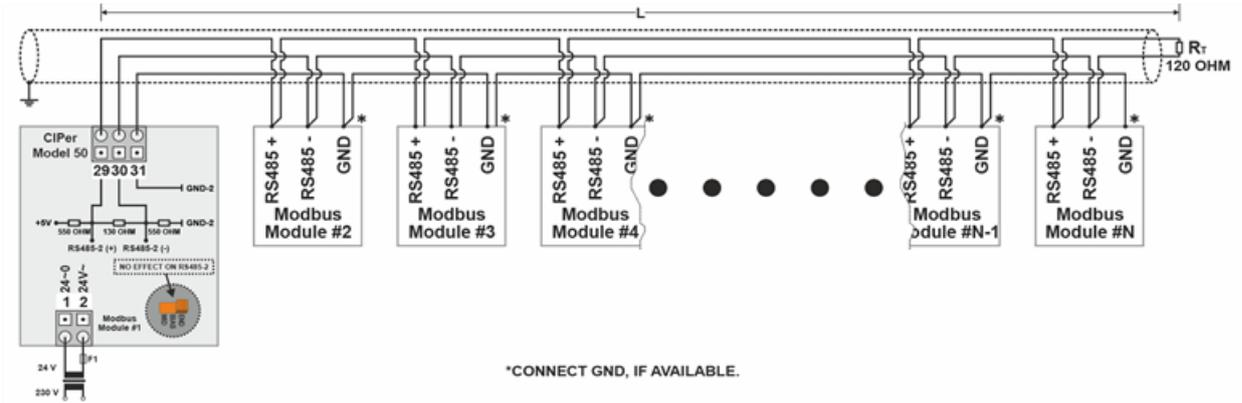
**Figure 51: Connection of an CIPer Model 50 Modbus master controller via its RS485-2 interface to a Modbus with slaves**
