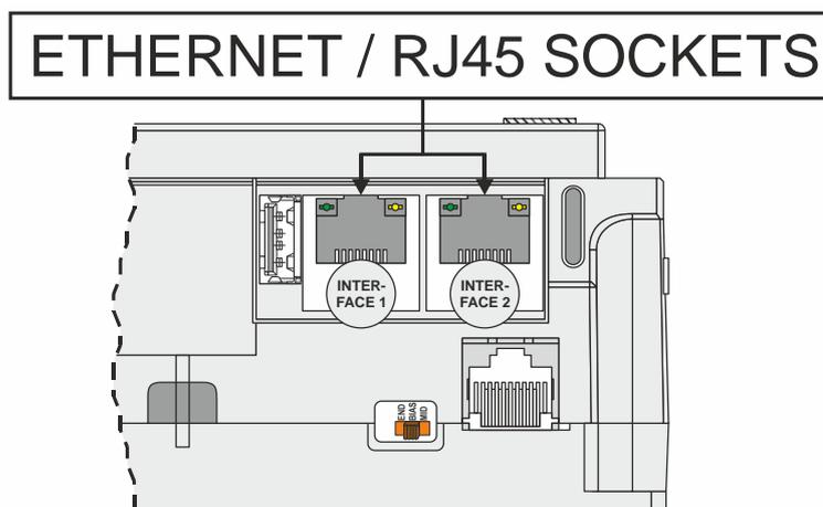
**Figure 8: Ethernet / RJ45 sockets**
