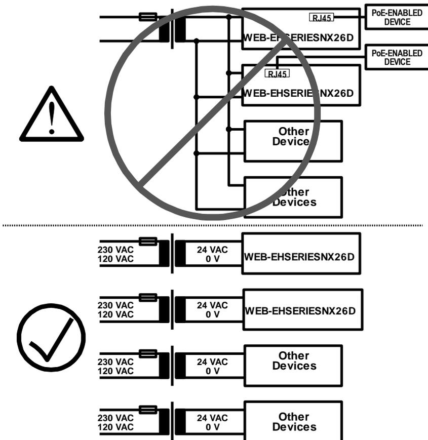
Figure 58: Connecting power to the PW M-Bus adapter
