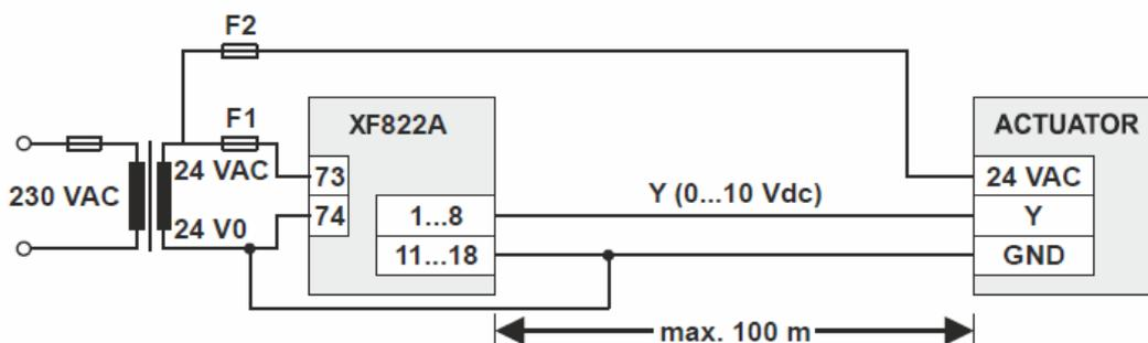
Figure 27: Power supply via Panel Bus I/O Module
