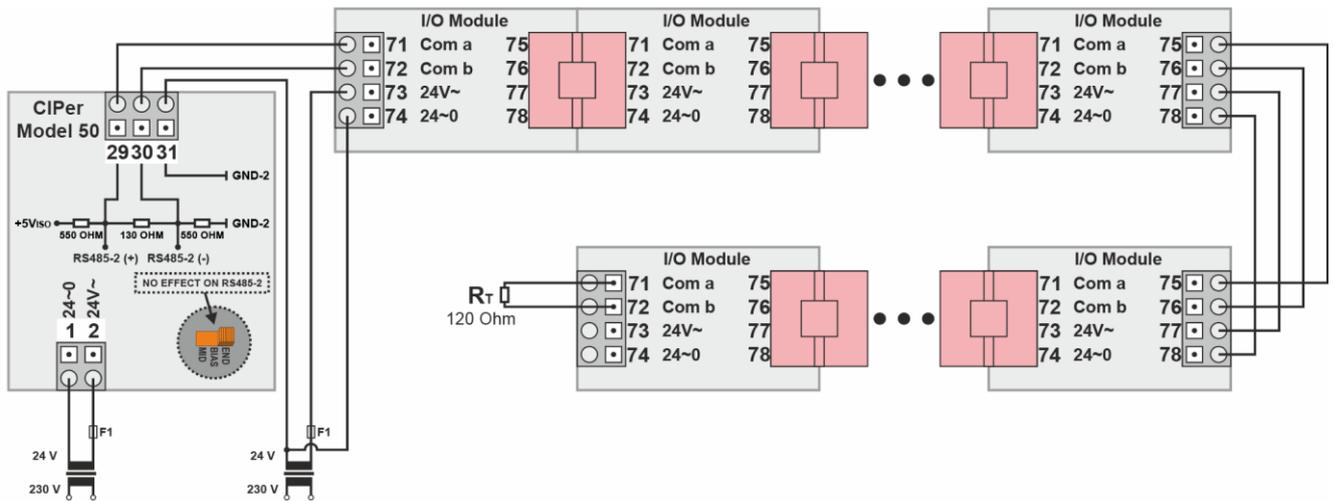
Figure 38: Connecting an CIPer Model 50 controller via its RS485-2 interface to a Panel Bus
