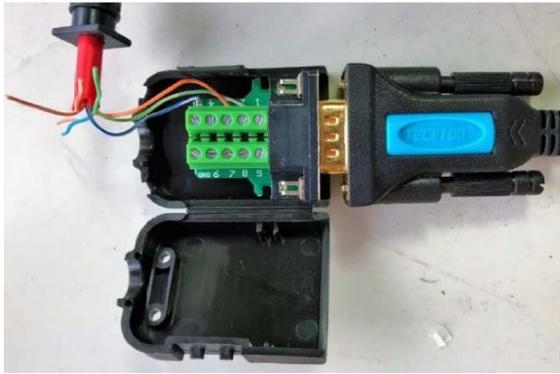
To can make up your own RJ-45 to conventional to RS-232 DB-9 female connecting cable using a standard Ethernet cable with the one end cut off. The standard color codes are:
