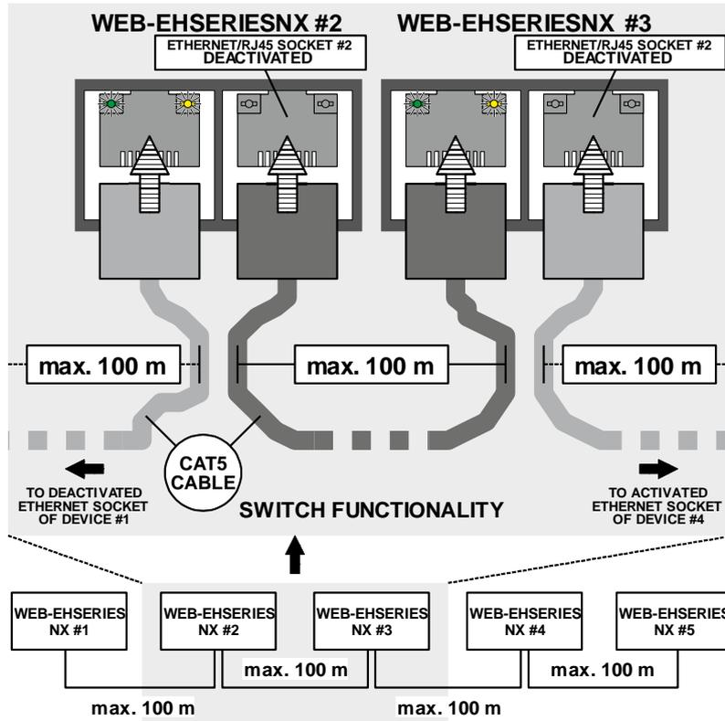
Figure 10: Allowed Ethernet wiring topology (“Switch functionality”)
