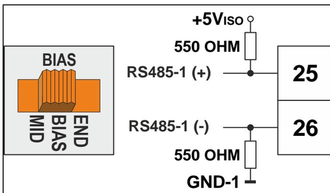
Figure 16: RS485-1 three-position slide switch setting BIAS
