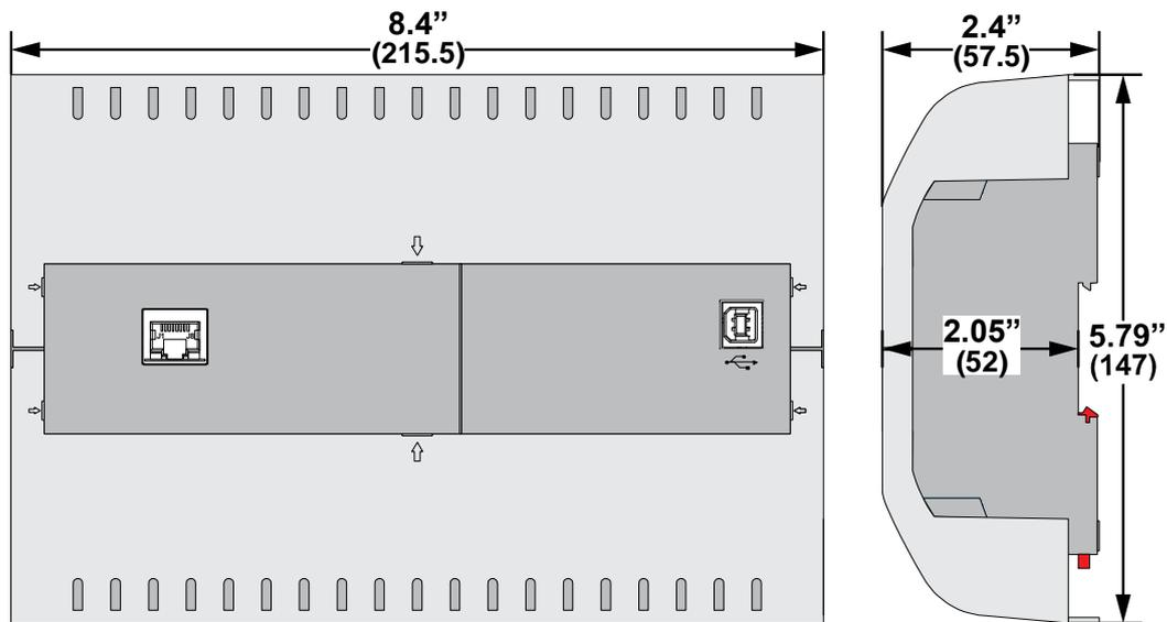
Figure 22: CIPer Model 50 controller with covers, dimensions in inches (mm)
