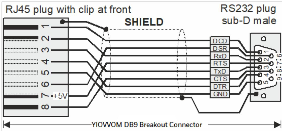
Figure 54: YIOVOM DB9 Breakout Connector power / communication cable details
