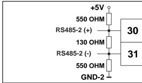
Figure 18: RS485-2 bias and termination resistors
