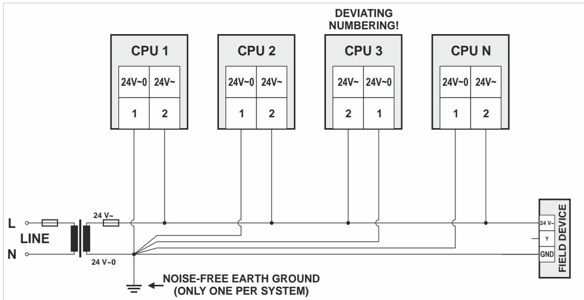
Figure 60: Connecting and earthing multiple CPUs
