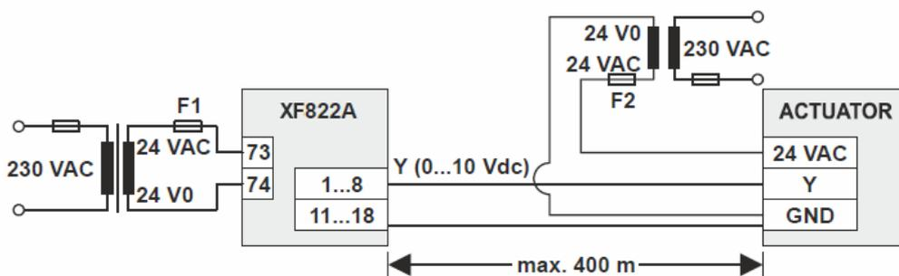
Figure 26: Power supply via a separate transformer
