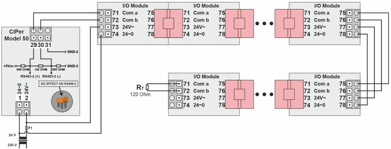
Figure 37: Connecting an CIPer Model 50 controller via its RS485-2 interface to a Panel Bus (single transformer)
