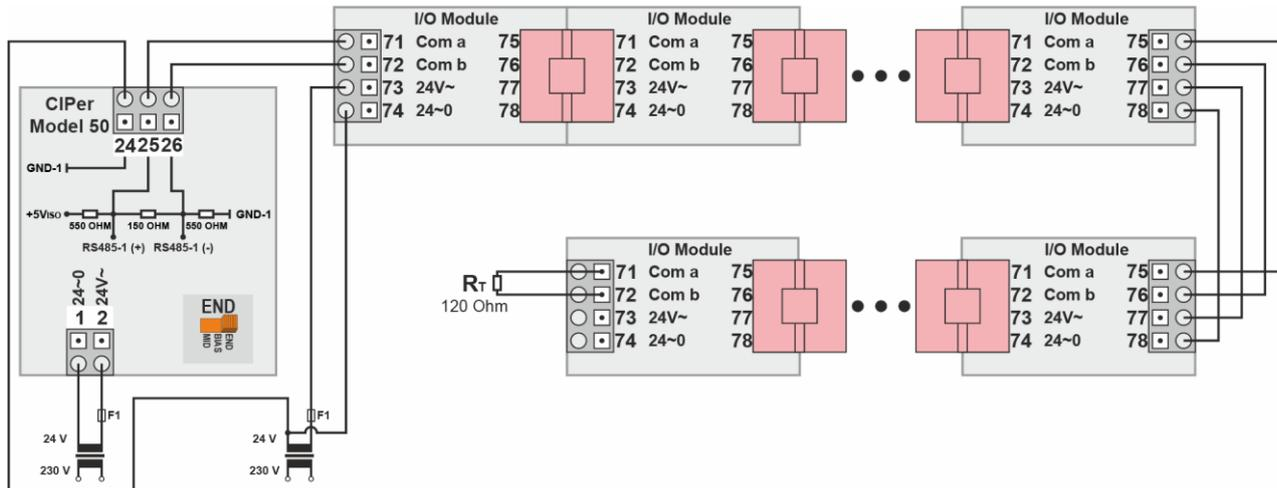
Figure 36: Connecting an CIPer Model 50 controller via its RS485-1 interface to a Panel Bus (two transformers)
