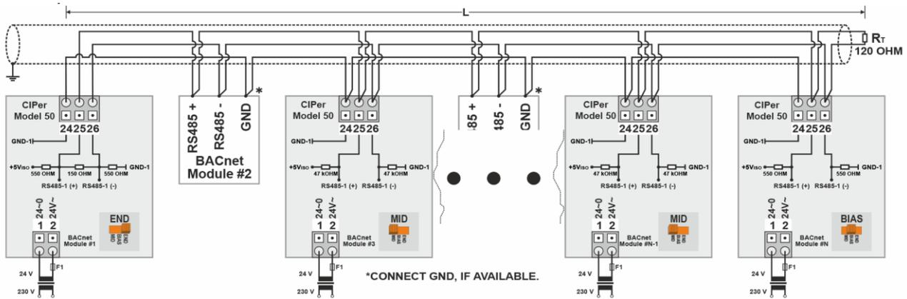
**Figure 47: Connection of multiple CIPer Model 50 controllers via their RS485-1 interfaces to a BACnet MS/TP Bus**
