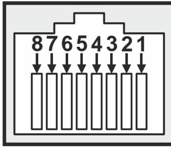
Figure 53: CIPer Model 50 RS232 / RJ45 socket
