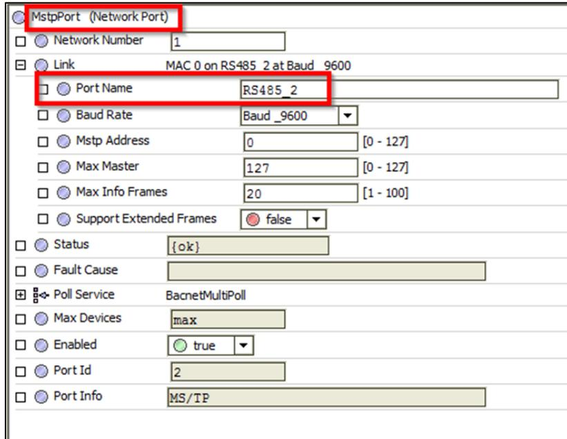
Figure 13: Configuring the RS485 interfaces in WEBs N4
