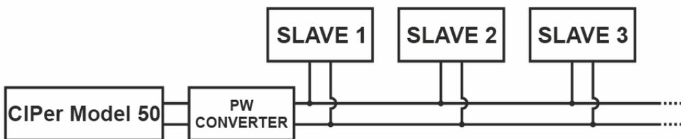
Figure 52: Allowed M-Bus wiring topology
