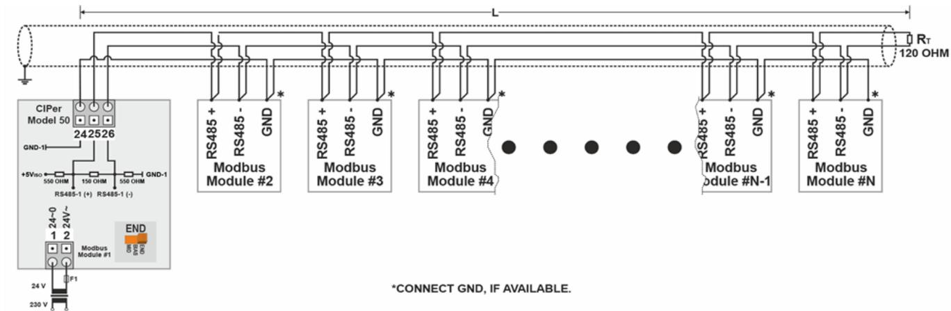
**Figure 50: Connection of an CIPer Model 50 Modbus master controller via its RS485-1 interface to a Modbus with slaves**
