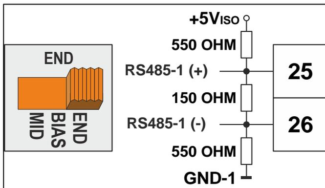
Figure 17: RS485-1 three-position slide switch setting END
