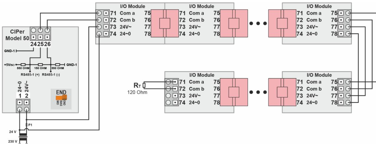
Figure 35: Connecting an CIPer Model 50 controller via its RS485-1 interface to a Panel Bus (single transformer)
