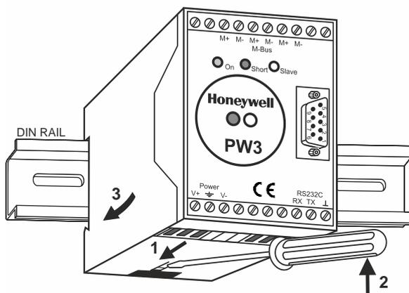
**Figure 55: Mounting of PW (PW3 shown here)**
