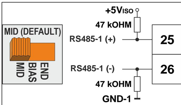
Figure 15: RS485-1 three-position slide switch setting MID
