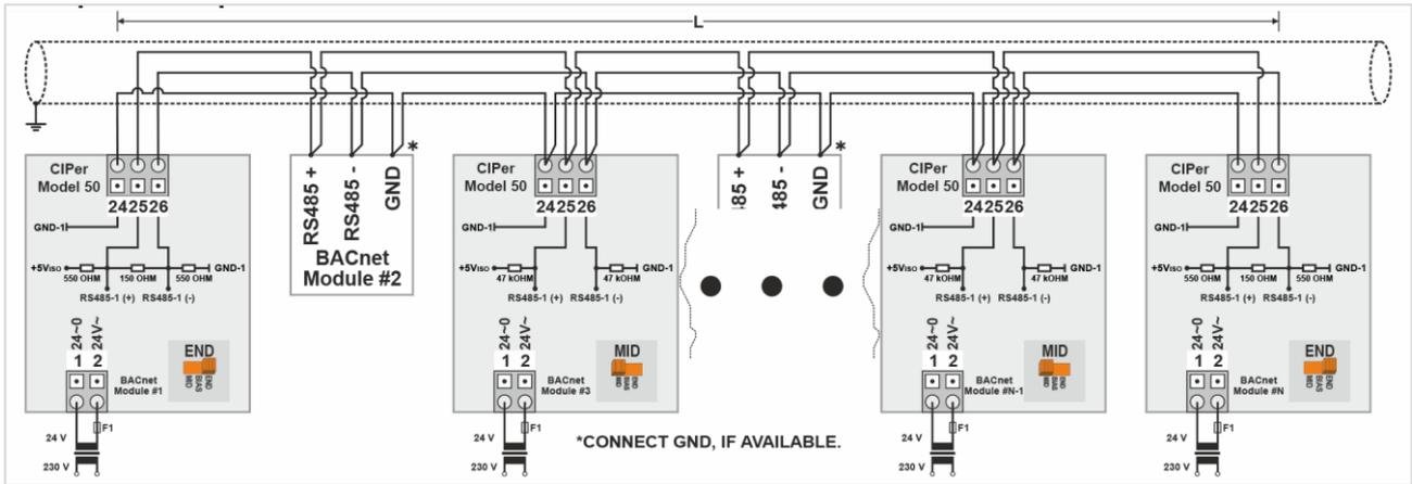
**Figure 46: Connection of multiple CIPer Model 50 controllers via their RS485-1 interfaces to a BACnet MS/TP Bus**
