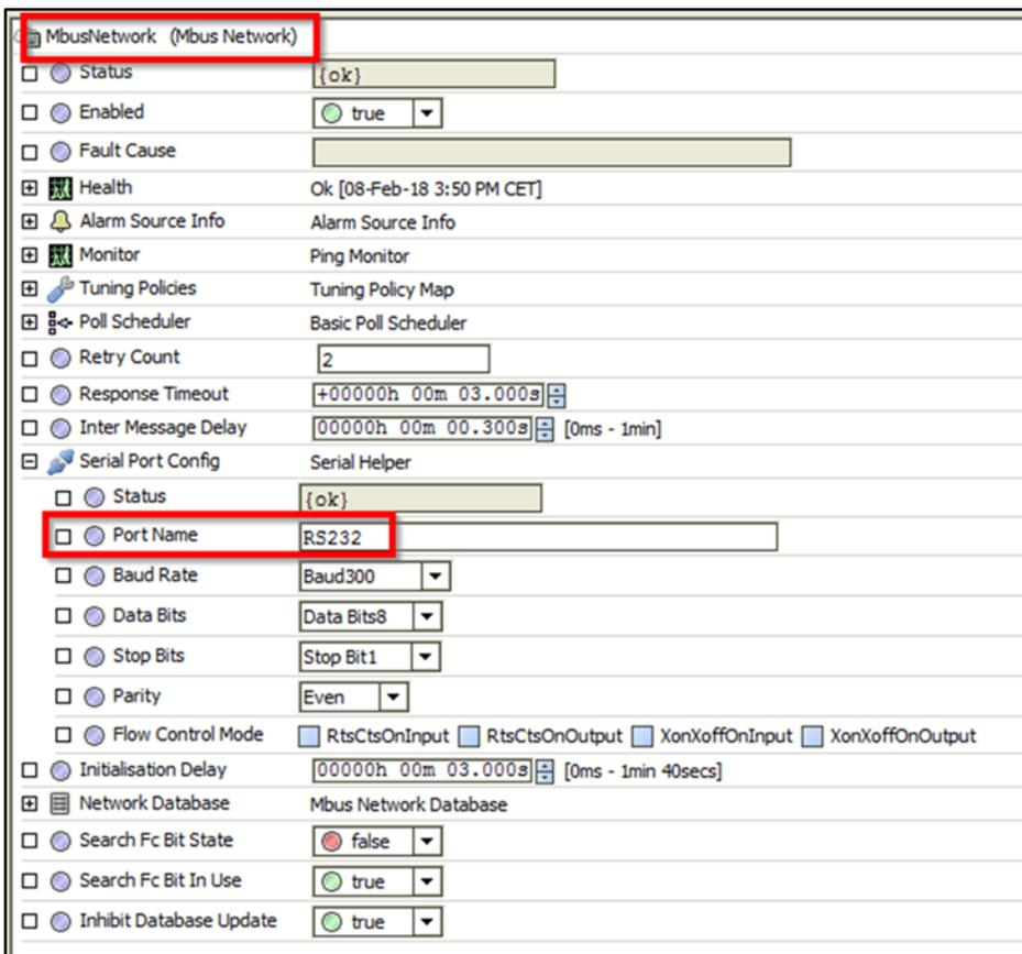
Figure 5: Configuring the RS232 Interface in WEBs N4
