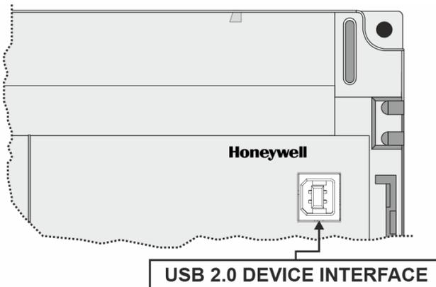
**Figure 7: USB 2.0 Device Interface**
