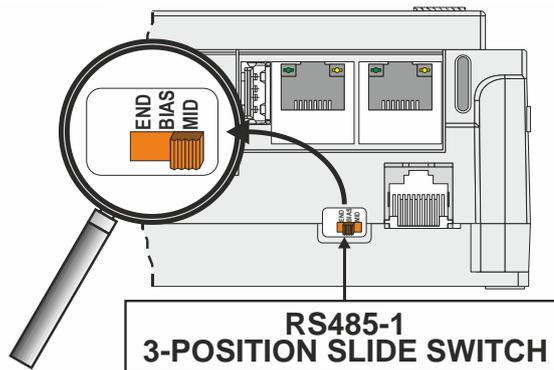
Figure 14: RS485-1 three-position slide switch
